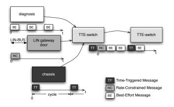
Fig. 1. TTEthernet in-vehicle sample application presenting the usage of the three traffic types.
