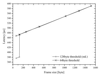
Fig. 5. Measurement results of standard configuration with 128 byte threshold in comparison with the modified configuration with 64 byte threshold.
