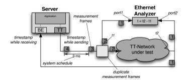
Fig. 6. The test setup for approach validation with an Ethernet performance analyzer.
