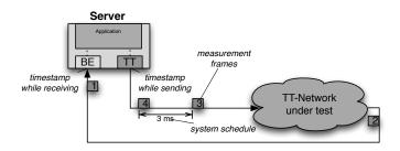
Fig. 4. The test setup of the used example measurement consists of a 3ms cycle.
